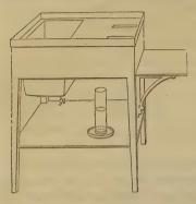
be made in the shelf, each about seven inches long, two wide, and one and a half deep. They should be placed with one of their narrowest ends about one inch and a half from the end of the shelf which is furthest from the well, and about eight inches apart. These depressions are to receive the beaks of retorts delivering gas into jars placed
